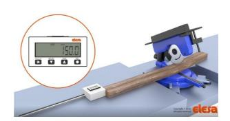
The MPI-R10 magnetic measuring device measures relative to a static frame-mounted magnetic band and plastic adhesive cover strip, with electronics housed in an IP54 or IP67 protected case making it suitable for fully manual or semi-automatic workstations even in dirty, wet environments. The measuring components are all contained in a hardwearing housing easily mounted on the workstation and allowing for quick replacement of the long-life lithium battery.
